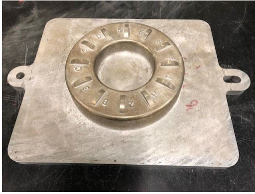
Figure 3. Matchplate drag pattern for the surface defect casting trial.
