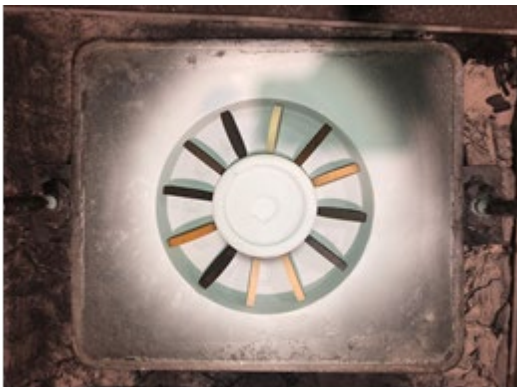
Figure 4. The disc-shaped specimens placed on the coreprints in the drag half of the mold.
