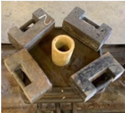
Figure 5. Chemically bonded sand mold fitted with sleeve ready for pour.
